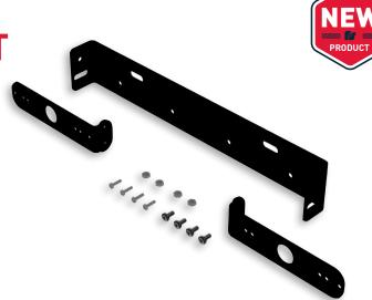
A new MicroPulse® license plate bracket is now available to order. This bracket allows (2) MicroPulse Ultra 3, MicroPluse Ultra 6, or MicroPulse C Series lights to be mounted horizontally to the upper or lower portion of the license plate. The light head mounting tabs can be oriented inwards or outwards to adjust for available space around the license plate. The light head mounting tabs can also be adjusted to set the correct angle.
