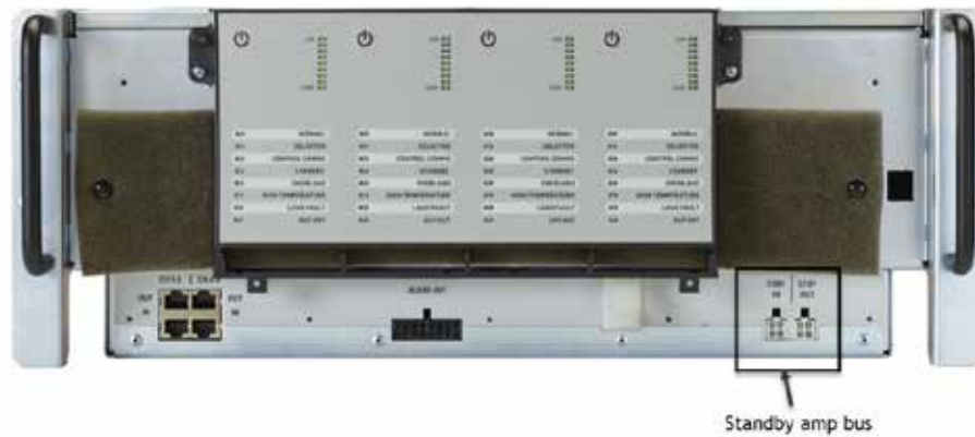
Figure 69 Standby amp bus ports on the Amplifier Chassis
