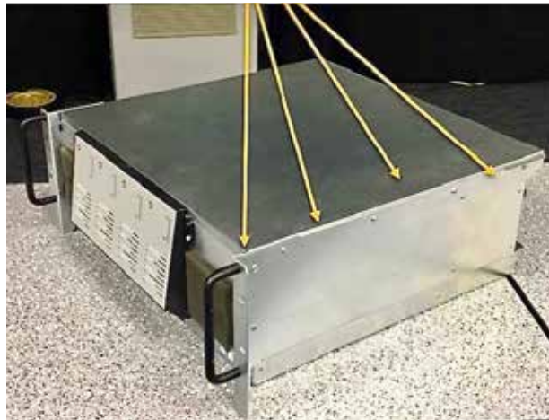
Figure 66 Removing the cover screws
