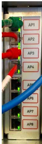
Figure 42 Internal AP Mux Card Connections
