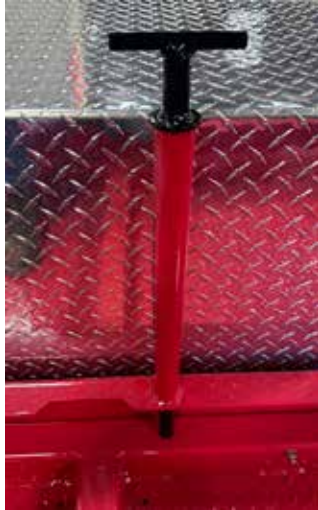
Figure 62 Verify pins are flush with tubes
