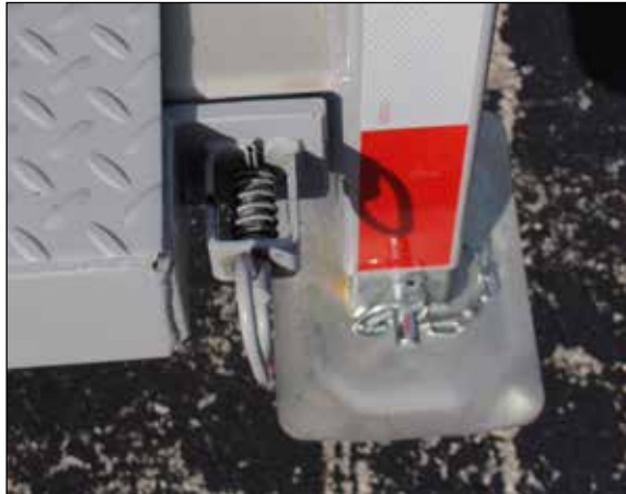
Figure 27 Spring-loaded safety latch
