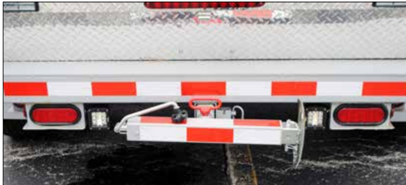
Figure 80 Back outrigger (#6) in the stowed position
