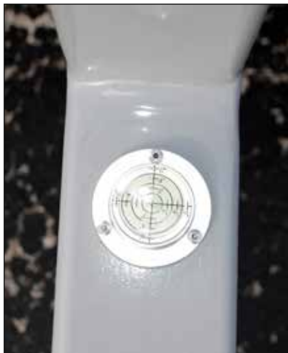
Figure 36 Bubble level centered
