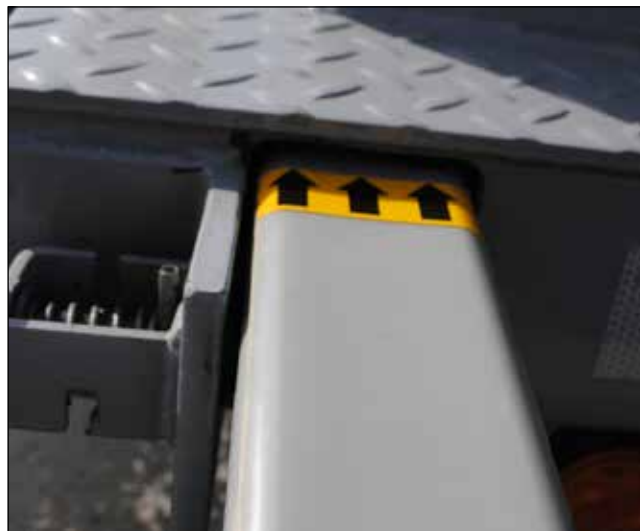
Figure 30 Outrigger Flush against the trailer
