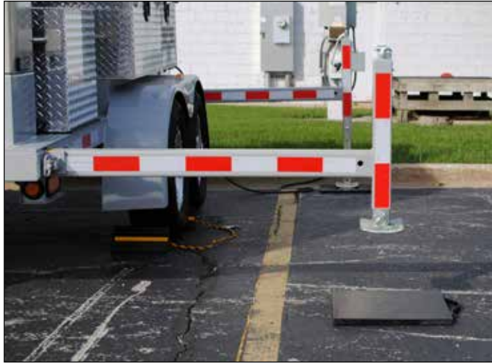
Figure 31 Support pad under the outrigger
