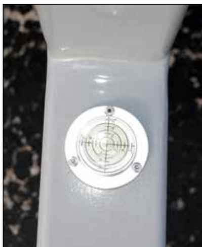
Figure 42 Bubble level centered
