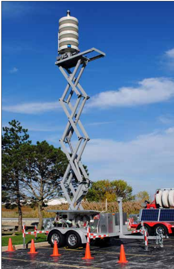
Figure 57 Siren fully raised without cables
