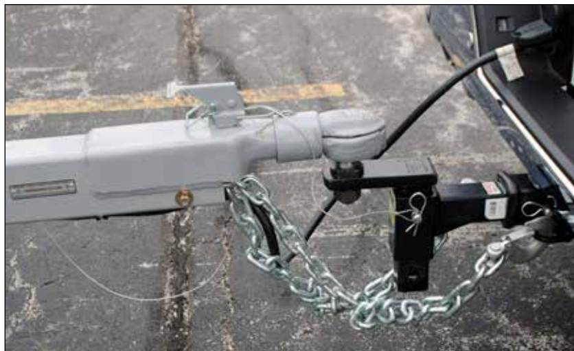
Figure 16 Breakaway cable connected to the tow vehicle
