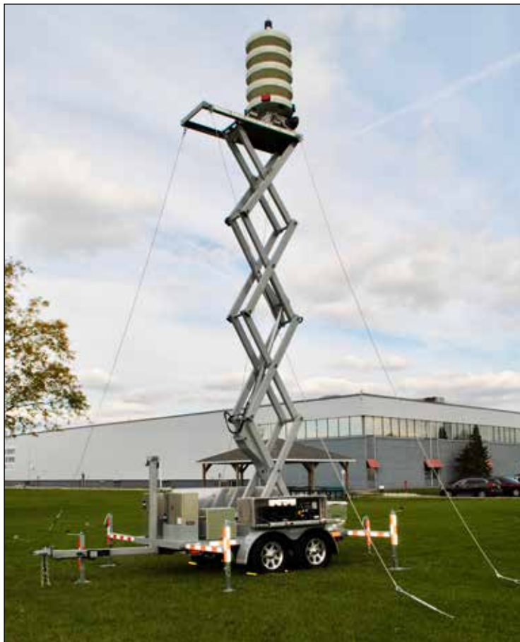
Figure 58 Siren fully elevated with cables
