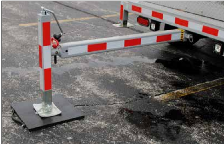
Figure 41 Support pad under outrigger #6
