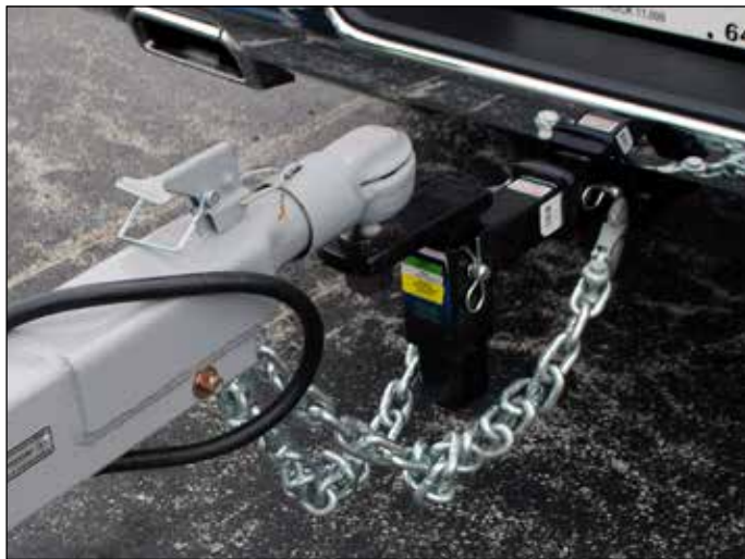
Figure 14 Safety chains attached to the tow vehicle
