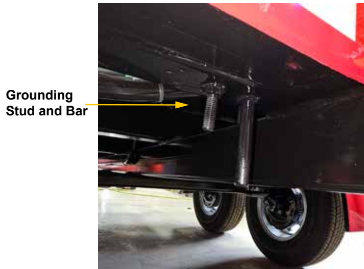
Figure 23 Location of Grounding Stud and Bar
