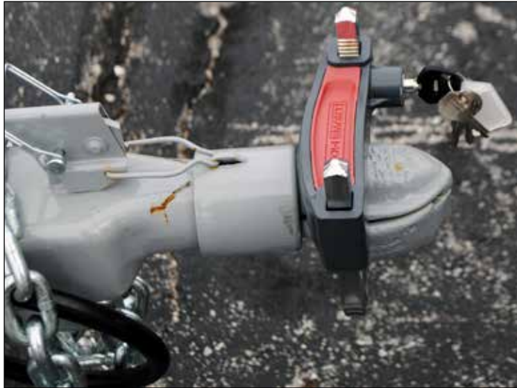
Figure 10 Coupler with lock
