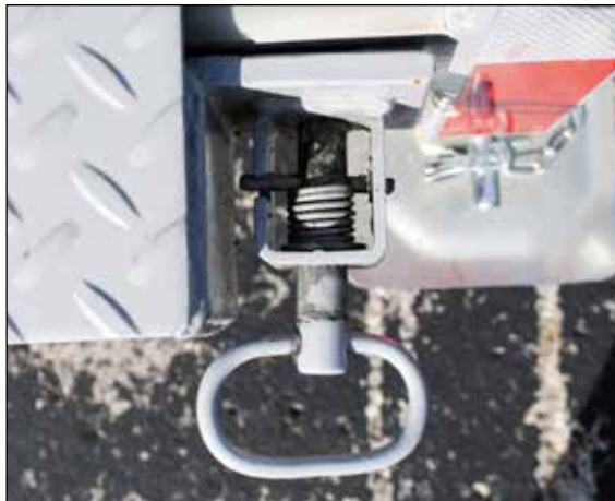
Figure 82 Spring-loaded safety latch rotated
