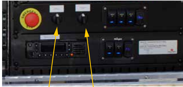
Figure 73 Lower/Raise siren head rotating switch
