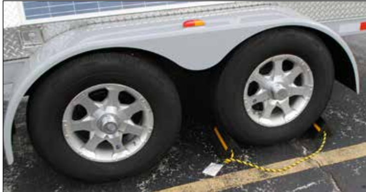
Figure 21 Wheel chocks in front and back of the tire
