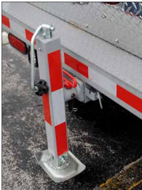
Figure 38 Spring loaded safety latch
