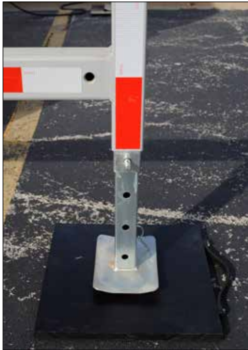
Figure 33 Leg lowered to the ground
