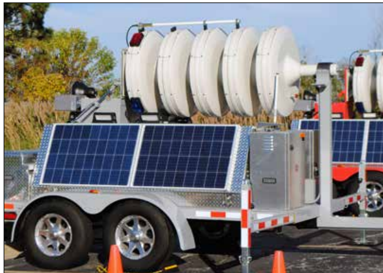
Figure 76 Siren in the stowed position
