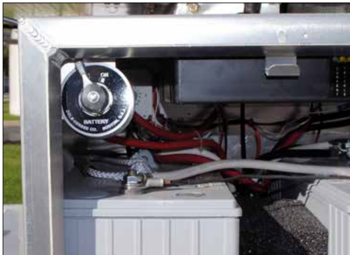
Figure 79 Siren master switch off
