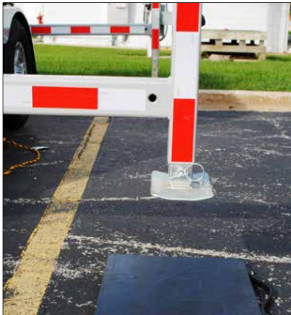
Figure 32 Locking pin unhooked
