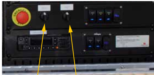
Figure 75 Toggle switch Down/Up siren head
