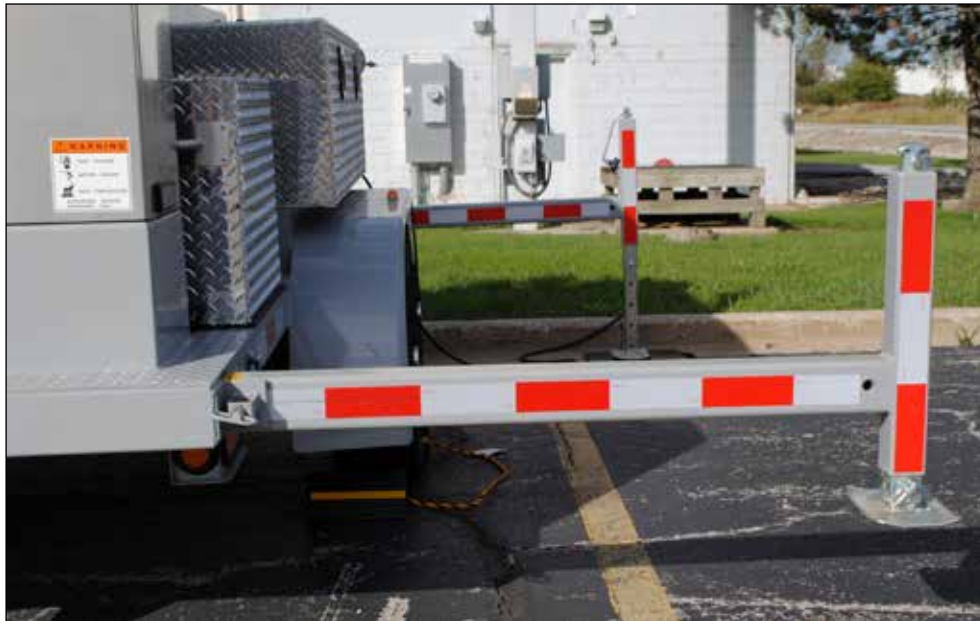
Figure 28 Pull outrigger outward to the marked stopping point
