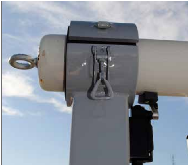
Figure 48 Siren's latch open
