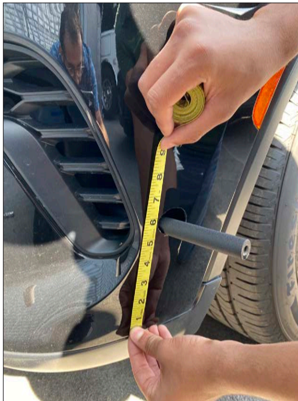
Figure 3 Pit bar hole location
