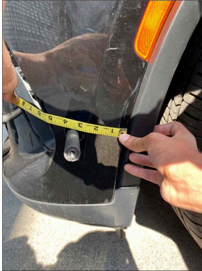
Figure 4 Pit bar hole location
