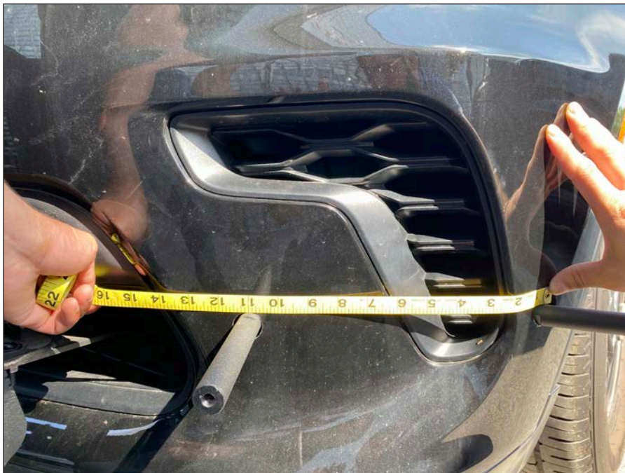
Figure 5 Pit bar hole location
