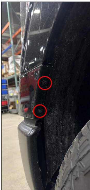
Figure 4 Front bumper upper cover trim panel fastener locations in wheel-well (Driver side shown)
