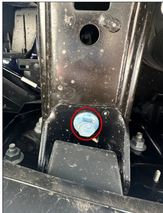
Figure 8 Rear tow hook to be removed (accessible from underneath the vehicle)
