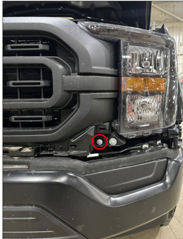
Figure 6 Grille shutter mounting bolts to be removed (Driver side shown)
