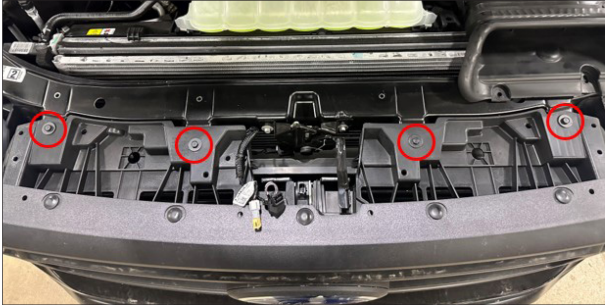
Figure 5 Grille fasteners to be removed
