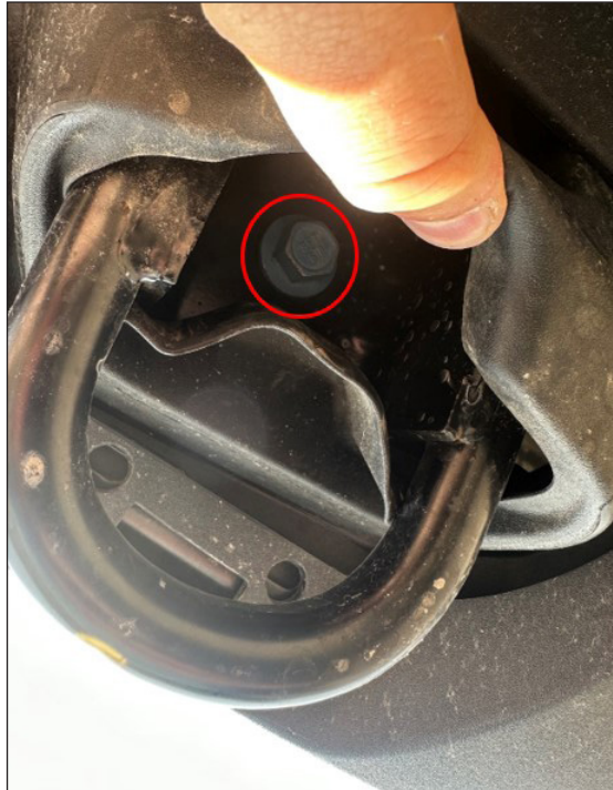
Figure 7 Front tow hook bolt to be removed
