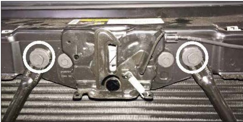
Figure 1 Bolts (circled) securing angled braces behind grille and front fascia
