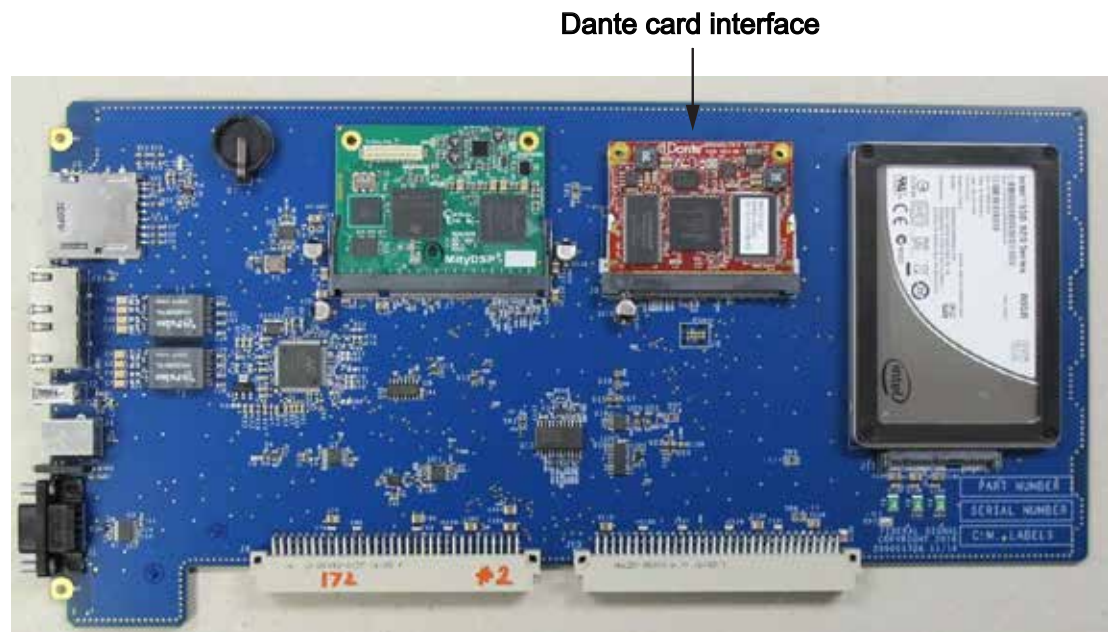
Figure 5 System Controller PCB that is Network Enabled (P-NET-G-IP)
