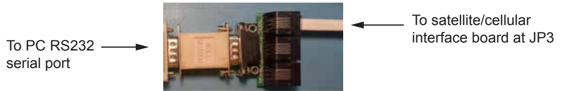
Figure 7 Modular data cable with the three-way adapter and null modem
